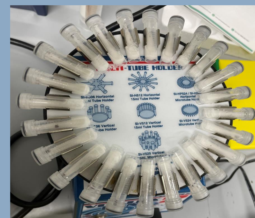
Fig 5: The bead bashing process breaks apart cells and exposes DNA needed for gene sequencing. This image shows 24 crushed beetle samples, along with lysis buffer, added to bead bashing tubes.
