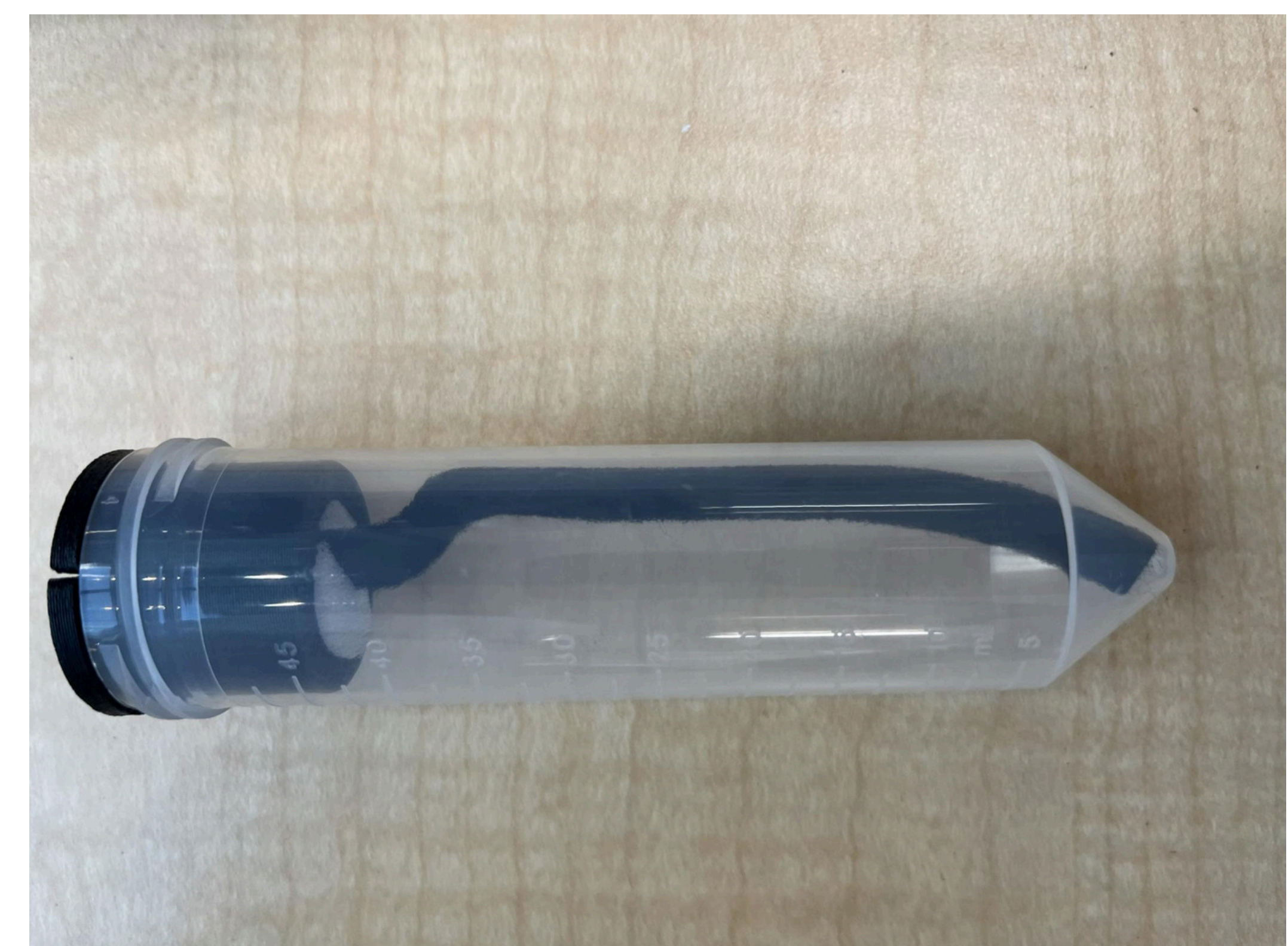
Figure 3: One module of the hydroponics growth system; a 50ml tube with a growth wick set into a urethane plug and a 3D printed collar.
