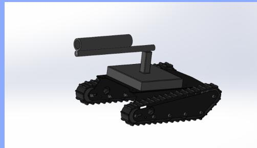
We used SolidWorks to visualize and refine our concept for the automated fire blanket deployment robot. By creating detailed 3D models and simulating various scenarios, we were able to test the robot's mechanisms and ensure its functionality. This process helped us develop a robust prototype that meets our goals for enhancing fire safety and providing first aid support.
