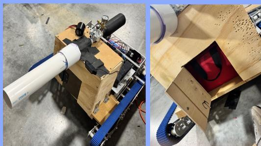
Our prototype features a pneumatic cannon designed to rapidly deploy fire blankets in emergency situations. The cannon ensures quick and accurate blanket deployment to contain and extinguish flames effectively. Additionally, the robot includes a compartment housing a first aid kit, providing immediate access to medical supplies for treating injuries. This combination of fire suppression and first aid capabilities enhances overall safety and emergency response efficiency.
