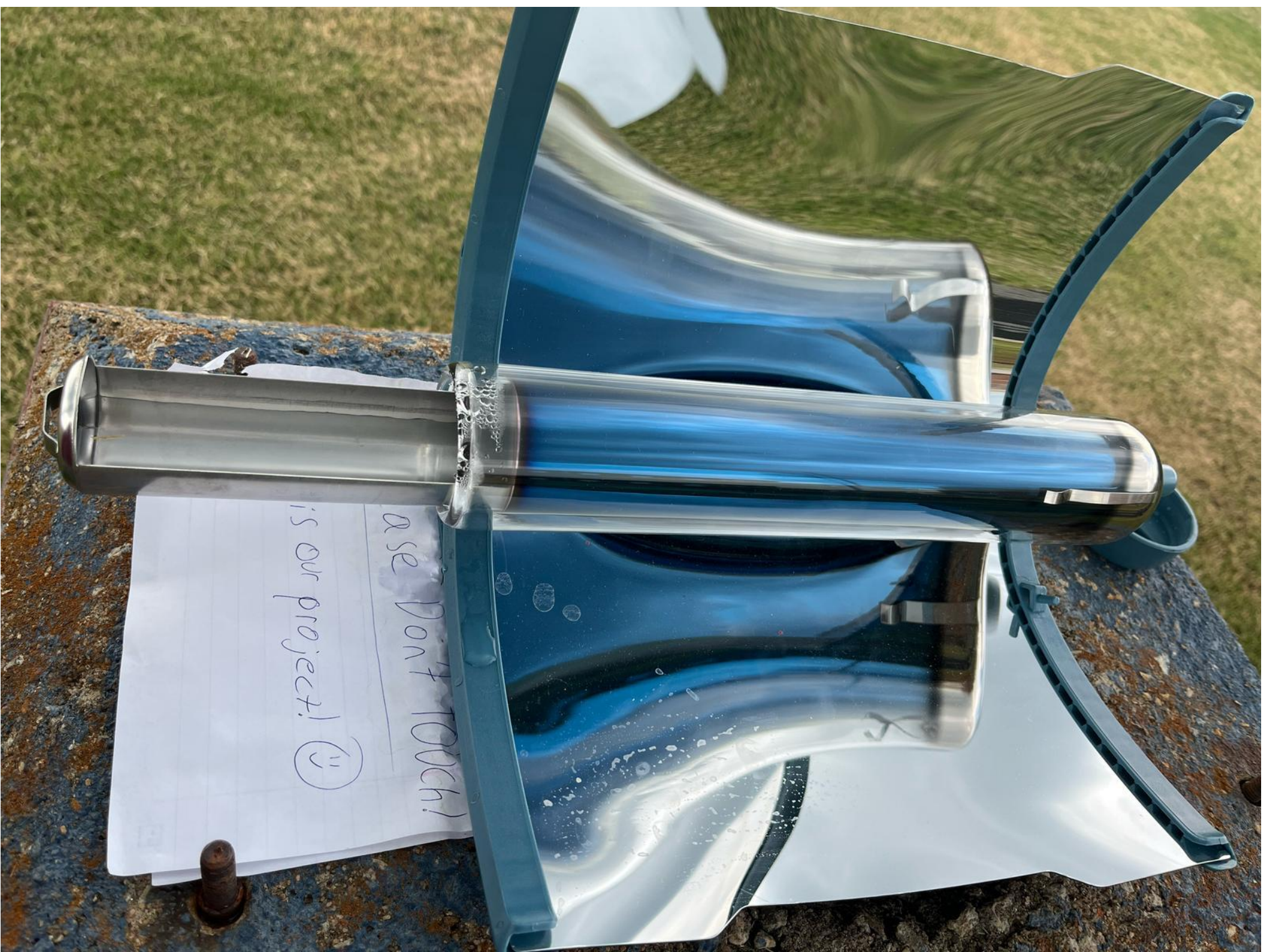
Figure 3: The final prototype during the experiment. Water goes in the metal sleeve then slides in the tube. Light is focused onto the tube using the mirrors.
